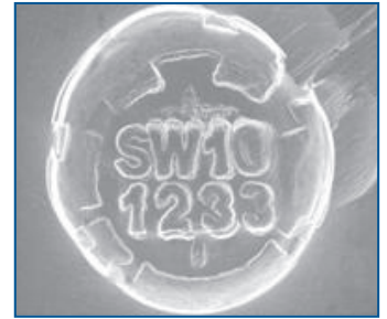
Example of a cartridge microstamped with specific information identifying the gun
